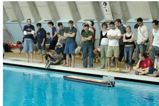
Figure 3. Second project in MECH 223 – students built cargo vessels to transport bulk cargo across a pool using pressurized soda bottles as the energy source.
